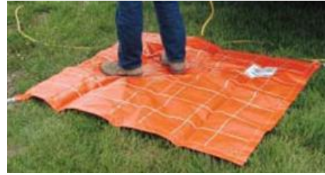
Figure 3: Equipotential grounding mat.
