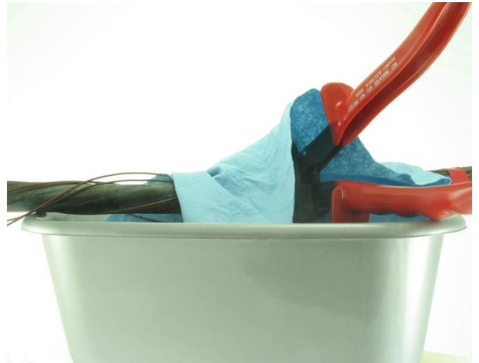
Figure 3: Absorb fluids with a rag.
