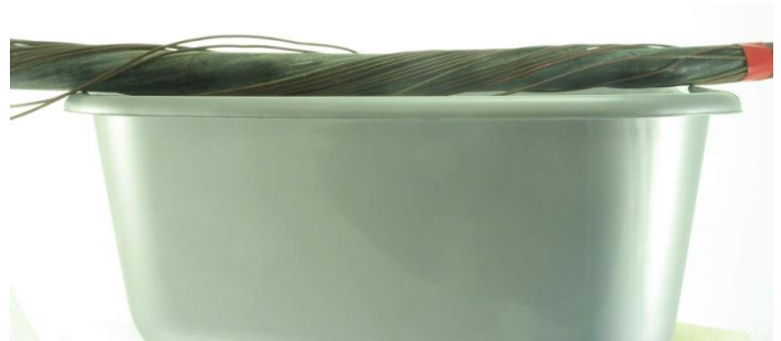
Figure 1: Place a basin under the cable to catch leaking fluids.
