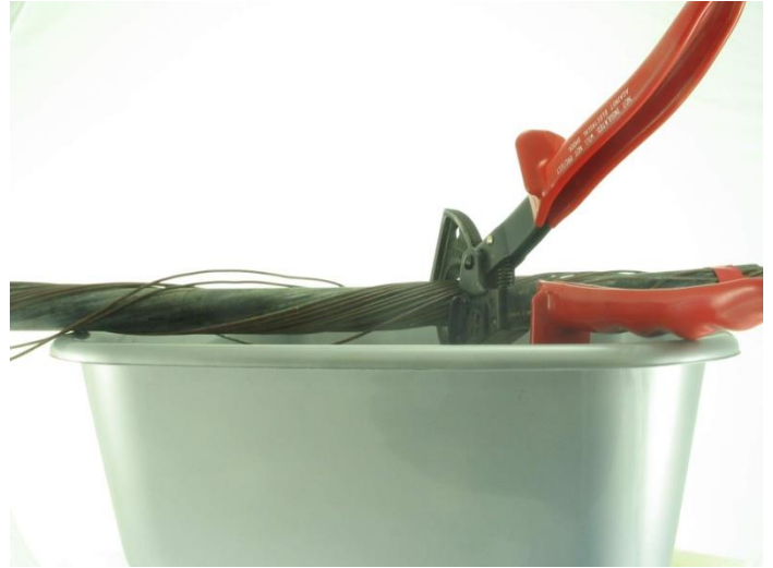
Figure 2: Position the spiking tool or cutters.
