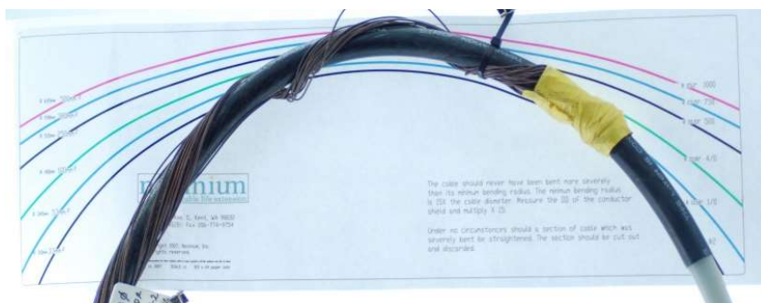
Figure 2: The 1/0 cable is bent more severely than its minimum bending radius.
