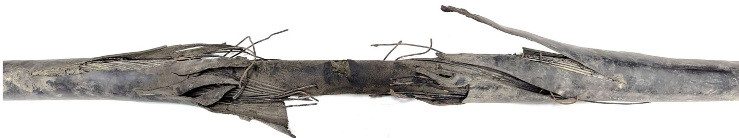
Figure 3: Failure sample of a midspan fault including additional length of unfaulted cable.
