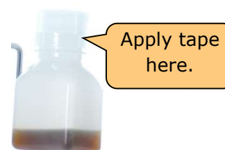
Figure 5: Apply vinyl tape to prevent the cap from unscrewing.
