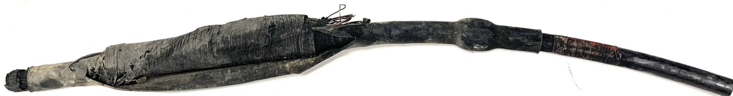
Figure 4: Failure sample of a faulted splice including additional lengths of cable and rejack kit.
