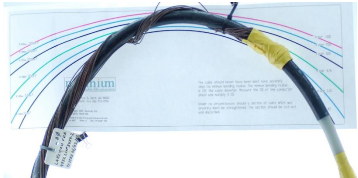
Figure 6: The 1/0 cable is bent more severely than its minimum bending radius.
