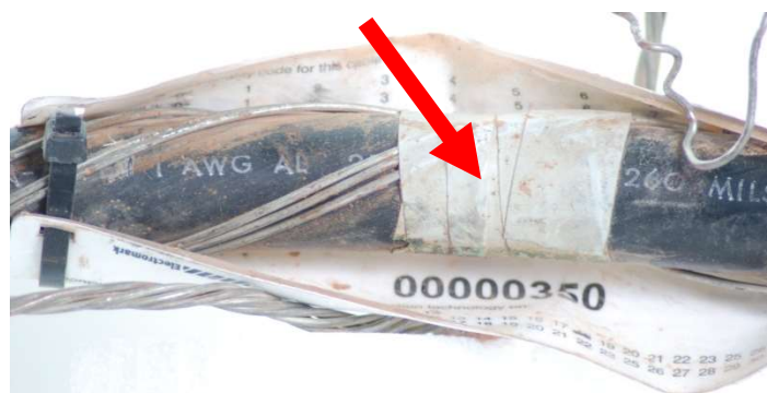
Figure 6: Bare neutrals secured with vinyl tape.
