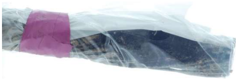
Figure 7: Sealed cable ends.
