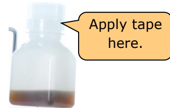
Figure 2: Apply vinyl tape to prevent the cap from unscrewing.
