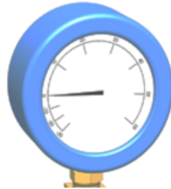
Figure 11: Perform a pressure test to test the cable system for leaks prior to injection.
