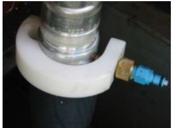
Figure 14: Connect the pump to the cable by using the injection adapter and connecting the QDs.
