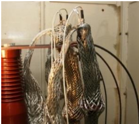
Figure 4: Use an ITD to streamline the TDR signal as it transitions into the cable.
