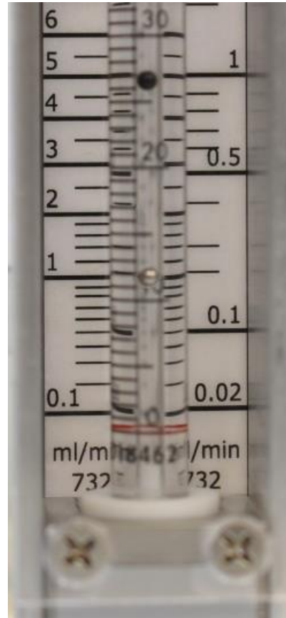
Figure 16: Liquid flow meter BBs are at 1cc/min.
