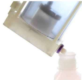
Figure 7: Transfer all fluids from the UP-RCVR tank to a graduated flush bottle.
