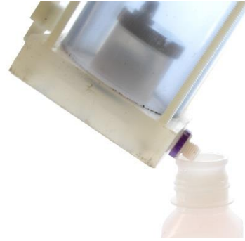
Figure 8: Transfer all fluids from the UP-RCVR tank to a graduated flush bottle.
