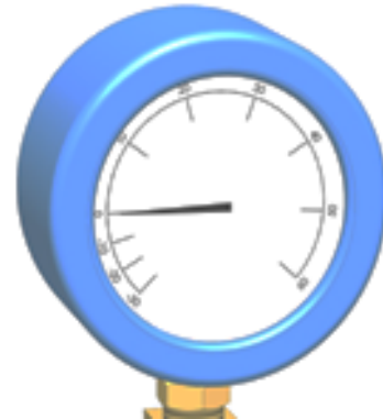
Figure 9: Perform pressure test to test the cable system for leaks prior to injection.
