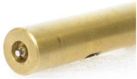
Figure 3: Insert the pin's tapered end first into the plug pin inserter tool.
