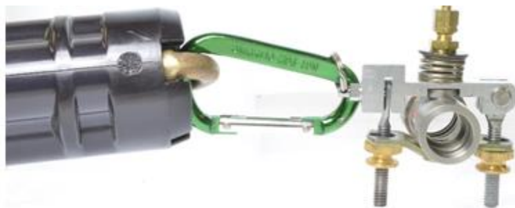
Figure 23: Remove using a hot stick.
