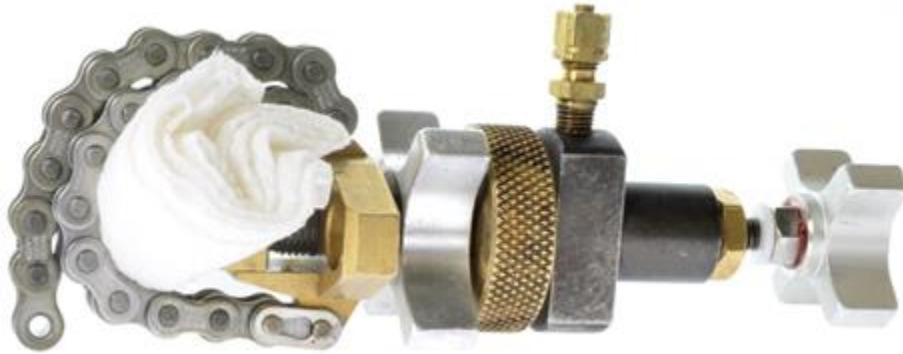
Figure 18: Use the chain and a paper towel to protect the gadget's tip.
