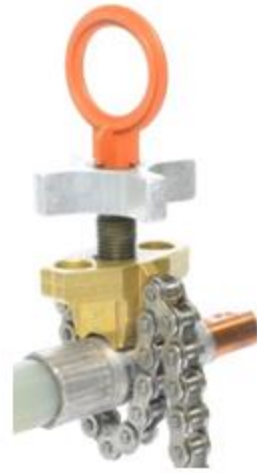
Figure 11: Hook the chain onto the saddle.
