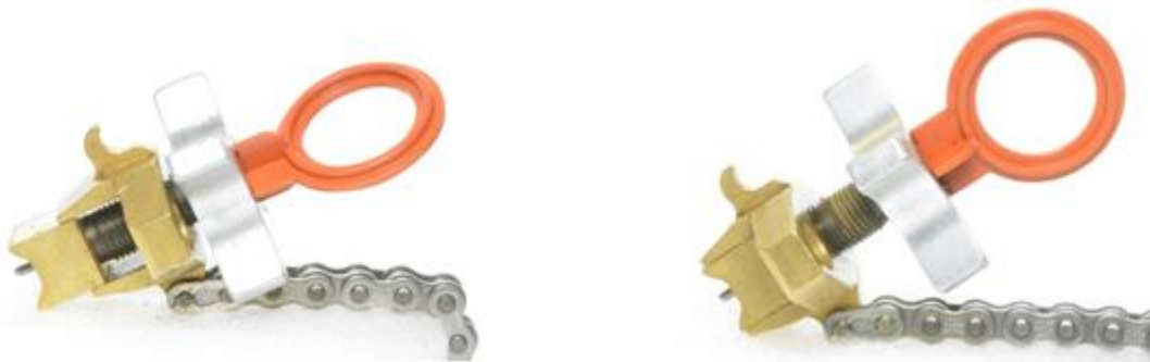
Figure 9: Wheel the brass block back and check for the pin tip.
