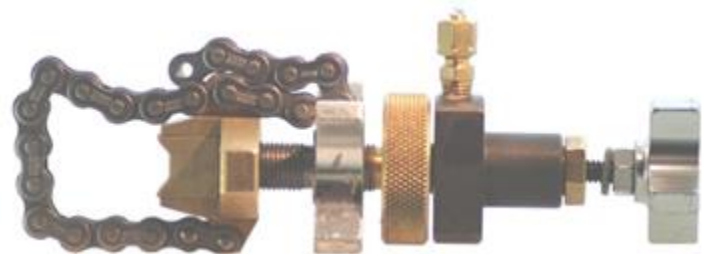
Figure 17: Hook the chain and partially thread the gadget.
