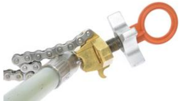
Figure 10: Seat the saddle onto the IA's injection hole.
