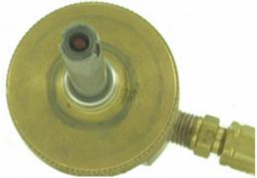
Figure 6: The colored tapered end of the plug pin is visible.
