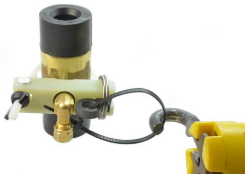
Figure 28: Remove using a hot stick.
