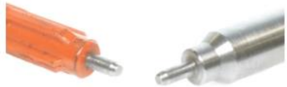
Figure 7: Examine the alignment pin’s tip for damage.
