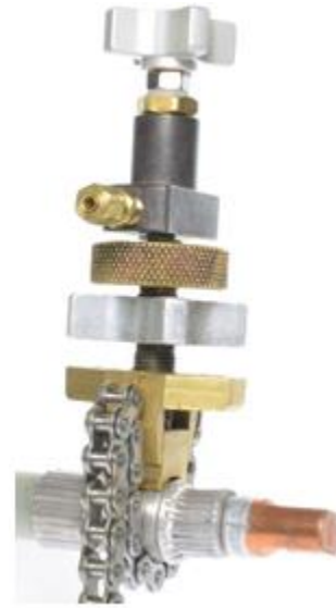
Figure 16: Turn the insertion knob to drive the plug pin in.
