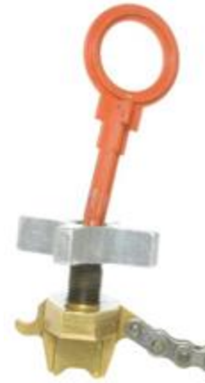
Figure 8: Alignment pin goes into the saddle.
