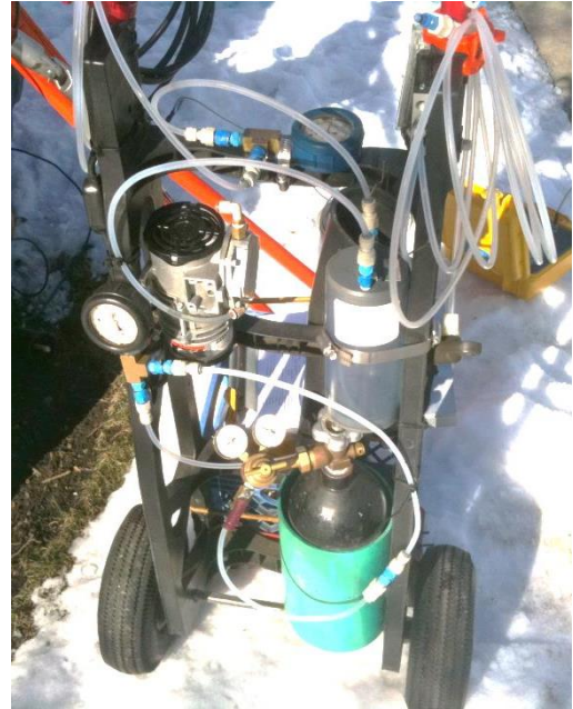
Figure 8: Possible configuration for the AC vacuum pump.
