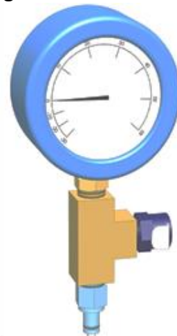
Figure 6: Use test gauge assembly to ensure adequate vacuum in the cable.
