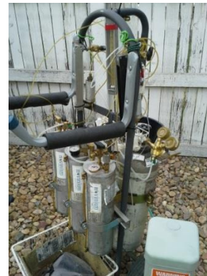
Figure 15: Tank secured to back of injection cart.
