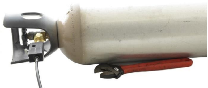
Figure 6: Lay the source tank on its side and invert slightly if the feed tank has no diptube
