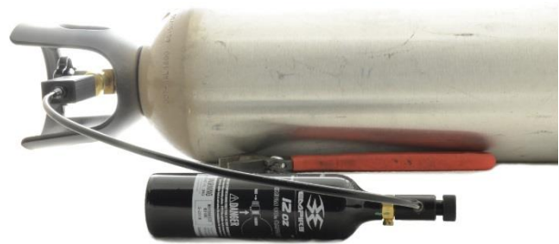
Figure 8: CO 2 bottle needs to be lower than the source tank.
