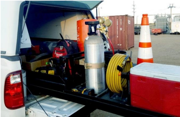
Figure 12: Secured tank with coil for easy storage and management of hose length.
