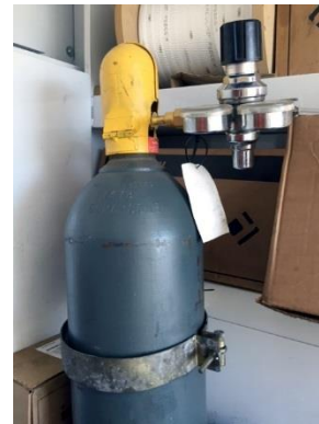
Figure 14: Clamps secure the tank for injection.
