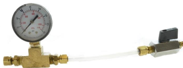
Figure 22: Inline gauge to verify pressure output from CO 2 tank.
