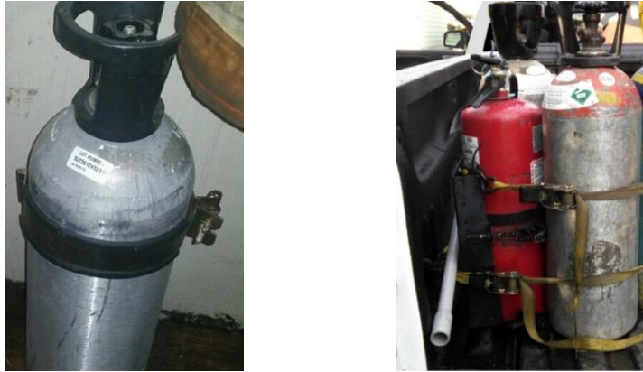
Figure 10: 20 pound cylinders secured for transportation with metal bands and nylon straps
