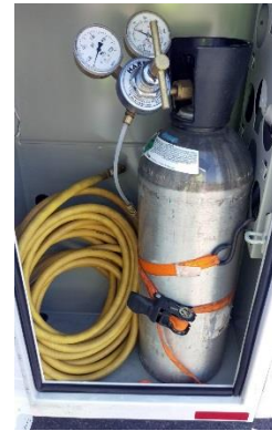
Figure 13: Secured in bay with hose on regulator.
