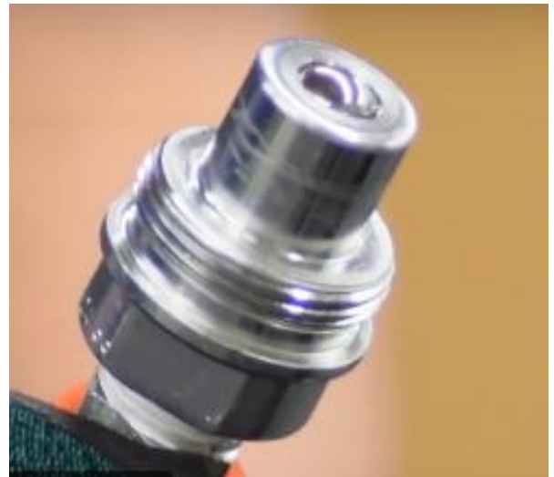
Figure 26: Make sure coupling are clean
