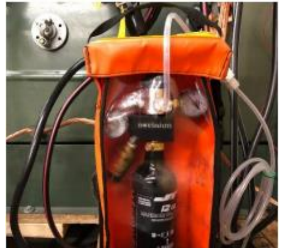
Figure 29: iUPR Regulator assemblies should be treated carefully in cold weather.
