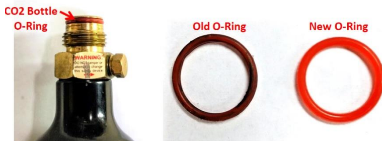
Figure 30: Replace bottle O-rings often to maintain a seal.
