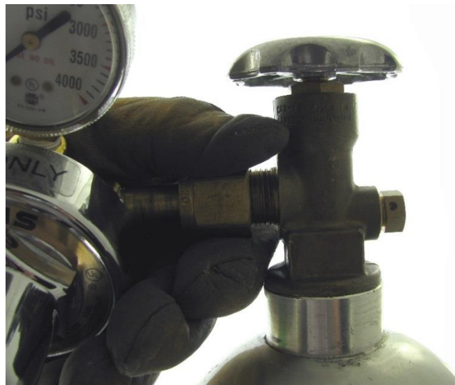
Figure 17: Thread the fitting onto the cylinder.
