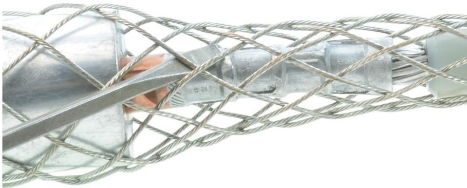
Figure 17: Use a screwdriver or squeeze to create a short between the Kellems grip and connector.
