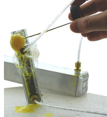
Figure 4: Using leak detecting fluid.
