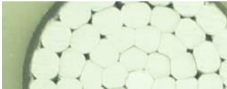
Figure 14: Tape shield leave gaps between strands.
