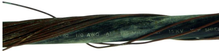
Figure 1: Look for writing on the cable jacket/outer layer.
