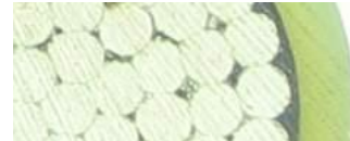
Figure 15: Extruded shields form around strands.
