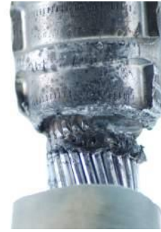
Figure 8: Damaged conductor strands.
