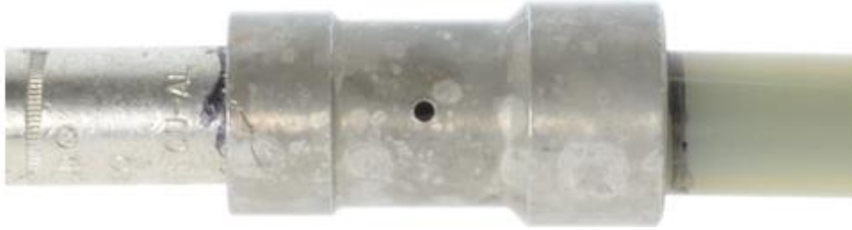
Figure 25: Quality check marks line up correctly.
