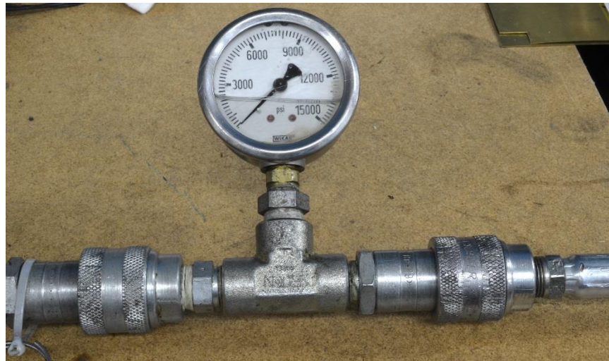
Figure 30: An example in-line hydraulic gauge between the swage press and foot pump. It must read at least 9000psi for a proper swage.
