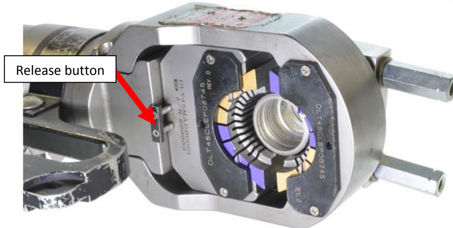
Figure 27: The release button is on the opposite side from the tool stop.
