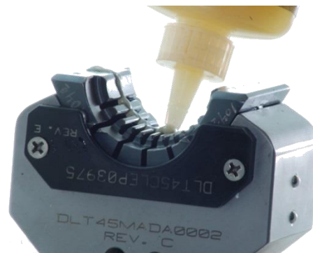
Figure 5: Add lubricant to the dies.
