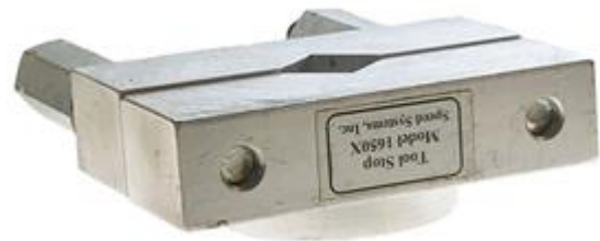
Figure 21: The rounded shoulder is down for large diameter cables.
