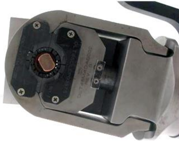
Figure 29: The swage head's shoulders have come completely together, fully compressing the swage die.
