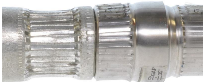
Figure 26: Crimp the connector as many times as possible.
