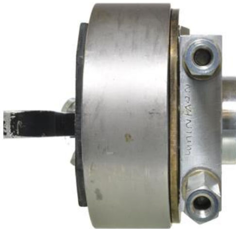
Figure 28: The swage head is square on the tool stop.
