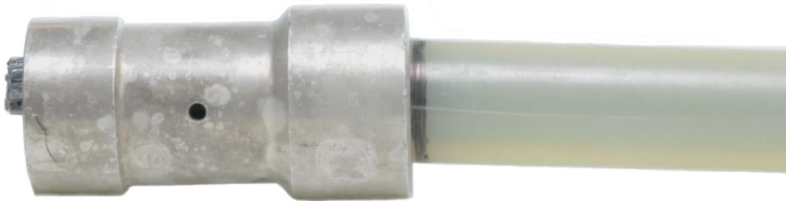
Figure 18: Use marks on the insulation to show full insertion into the IA.
