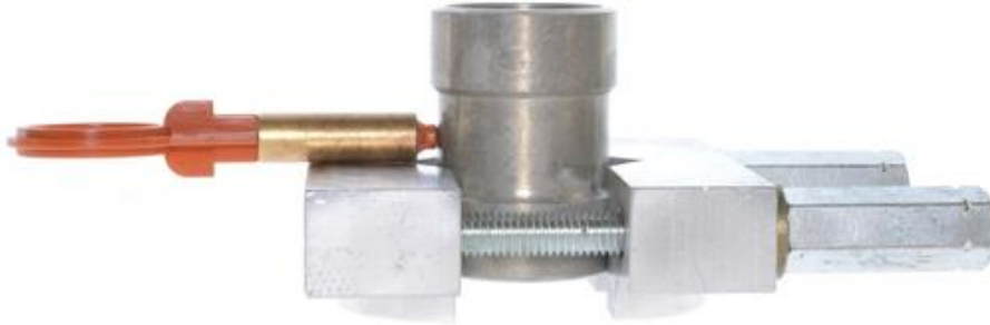
Figure 23: Bushing resting flush against tool stop.
