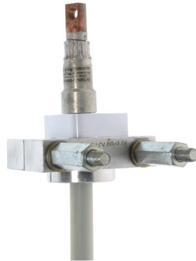
Figure 31: Spacing the tool stop with the V-spacer.
