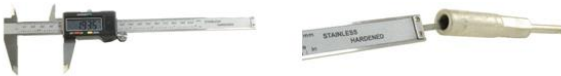
Figure 7: Measure the connector barrel depth with a digital caliper.
