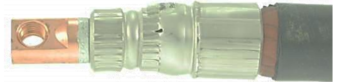
Figure 34: Improper swage on the IA's mid-section.
