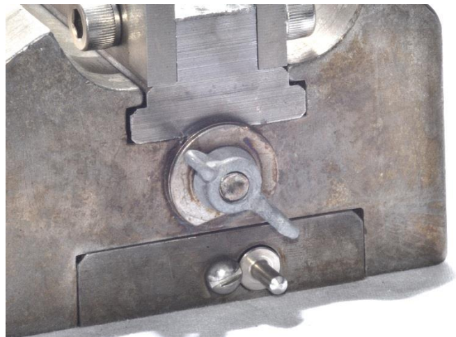
Figures 9 and 10: The washer that holds the blade block in.
