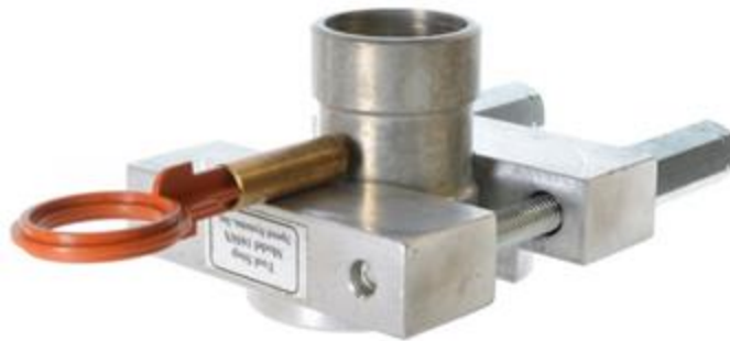
Figure 37: IA and pin rest in the tool stop.
