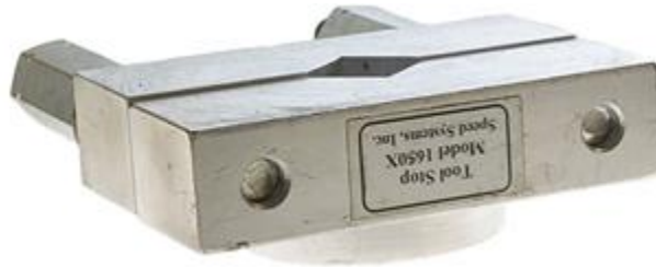
Figure 36: The rounded shoulder is down for large diameter cables.
