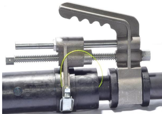
Figure 67: The bleed tube goes between the sleeve and the bus body.
