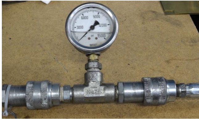
Figure 52: An in-line hydraulic gauge between the swage press and foot pump. It must read at least 9000psi.
