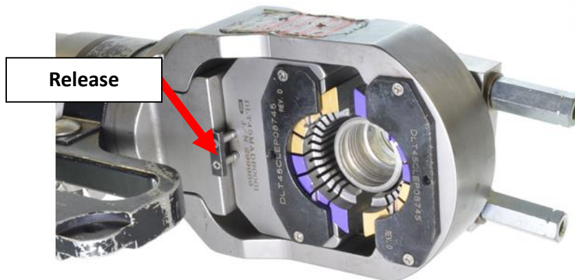
Figure 48: The release button is on the opposite side from the tool stop.
