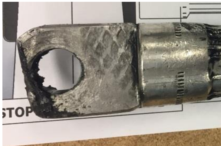
Figure 61: Any deformities on the mating surfaces can cause premature failures.
