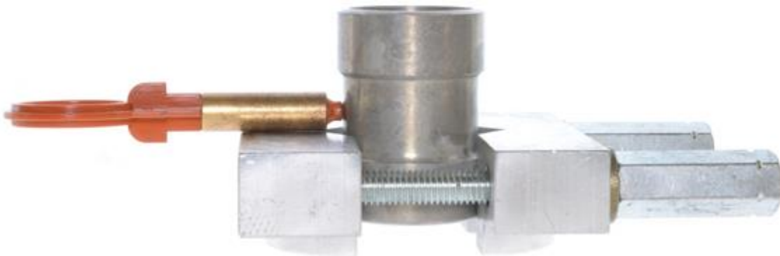
Figure 38: Bushing resting flush against the tool stop.
