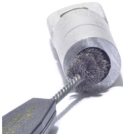
Figure 32: Wire brushing the connector
