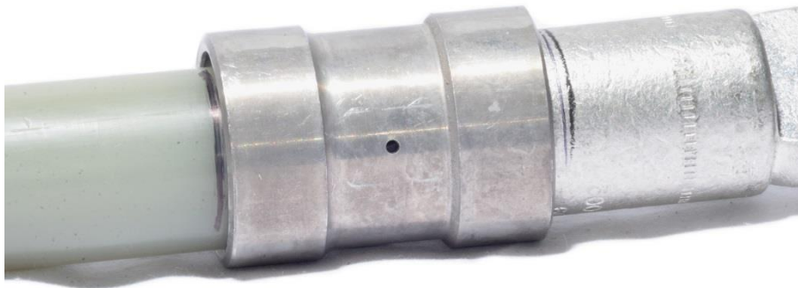
Figure 46: The QC marks above and below the edges of the IA.
