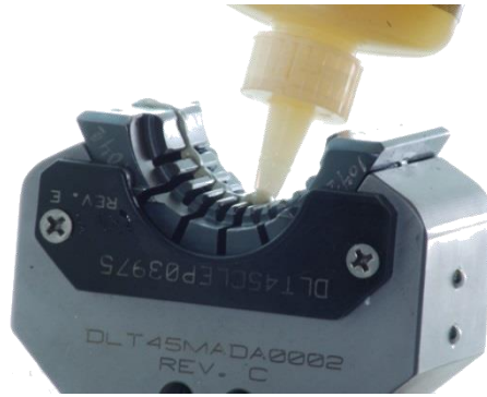
Figure 45: Add lubricant to the die.
