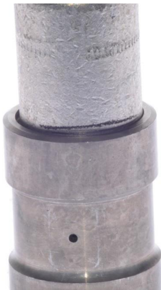
Figures 14 and 15: Mark the connector just above the edge of the IA to verify full insertion into the IA.
