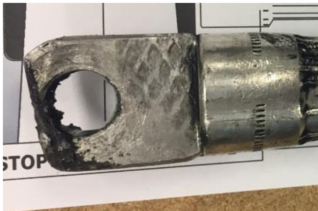
Figure 54: Any deformities on the mating surfaces can cause premature failures.
