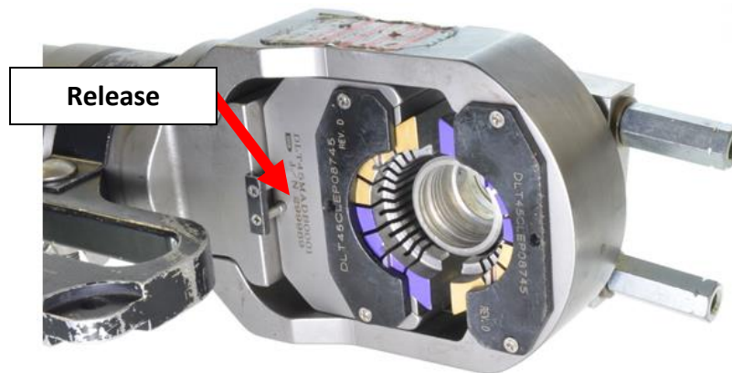
Figure 51: The release button is on the opposite side from the tool stop.
