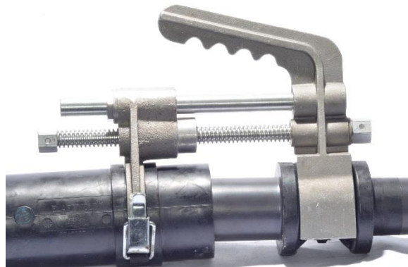
Figure 65: Place the installing tool on the components.
