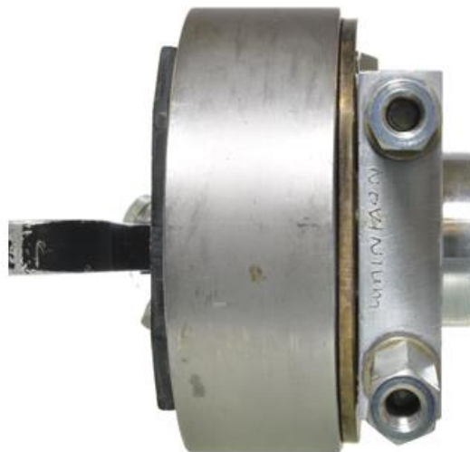
Figure 49: The swage head is square on the tool stop.
