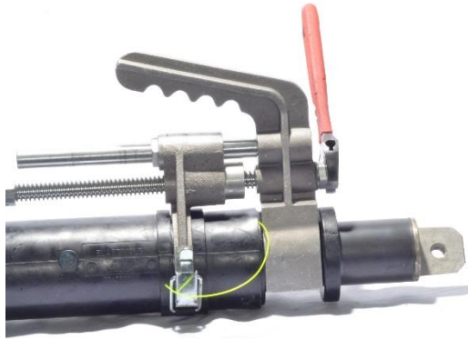
Figure 66: The sleeve installing tool can be run with a wrench on the hex bolt.
