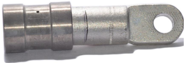
Figures 14 and 15: Mark the connector just above the edge of the IA to verify full insertion into the IA.
