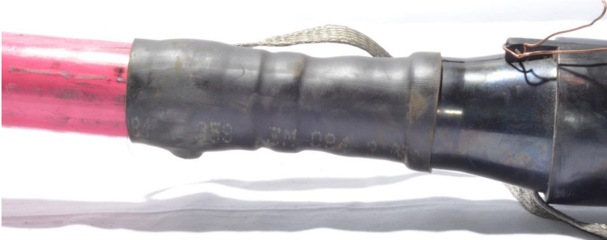
Figure 71: The water seal kit deployed on the cable adapter over to the cable jacket.
