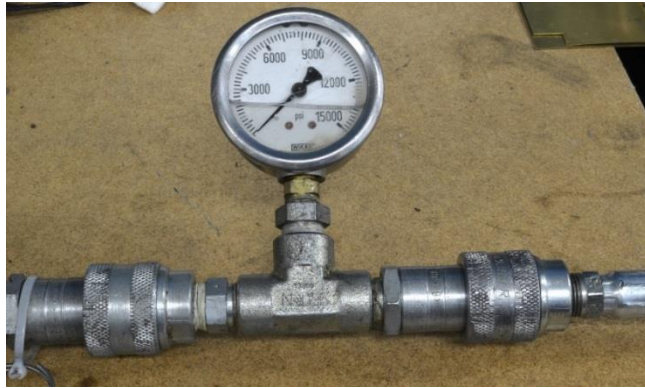
Figure 50: An example in-line hydraulic gauge between the swage press and foot pump. It must read at least 9000psi for a proper swage.
