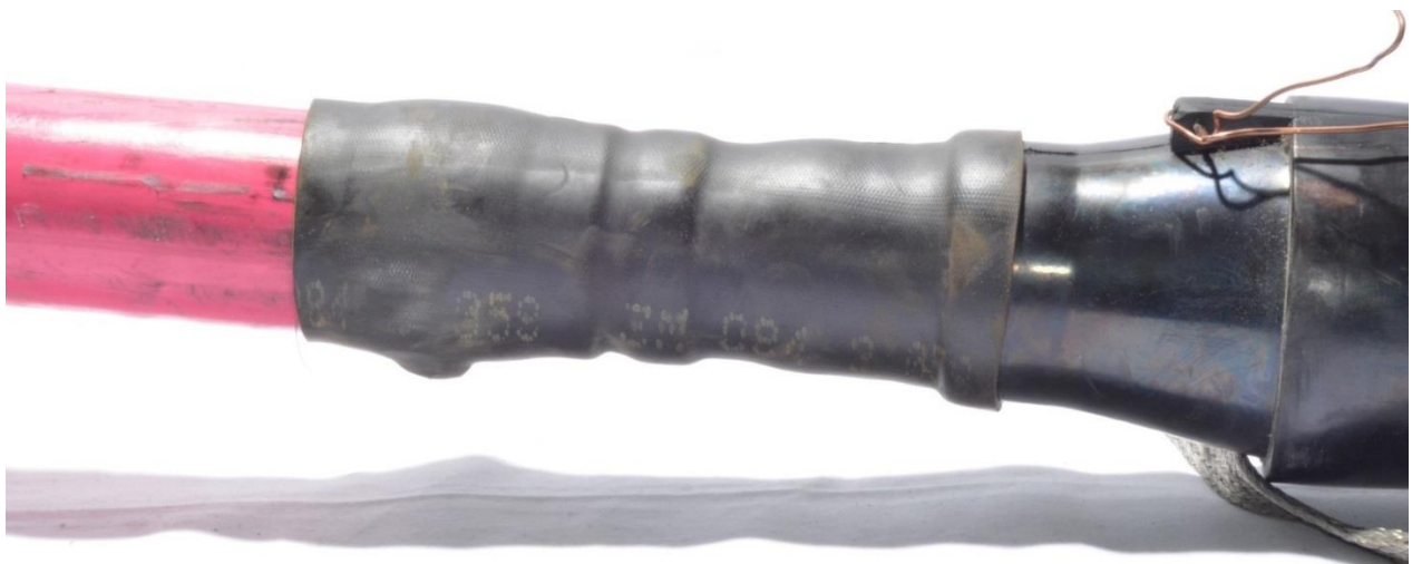
Figure 58: The water seal kit deployed on the cable adapter over to the cable jacket.
