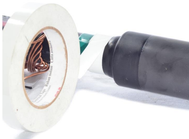
Figure 56: Wrapping the cable adapter can help to hold it in place.
