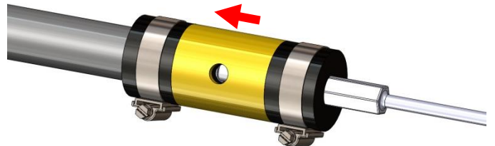
Figure 6: Slide the injection adapter over the terminal and tighten the hose clamps.
