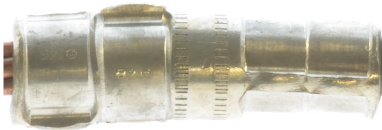
Figure 3: Place the maximum amount of crimps possible.
