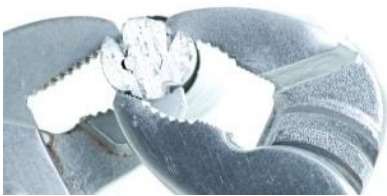
Figure 9: Pull the cut connector apart.
