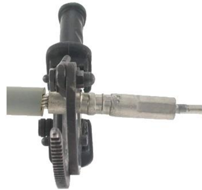
Figure 1: Cut next to the bottom crimp.
