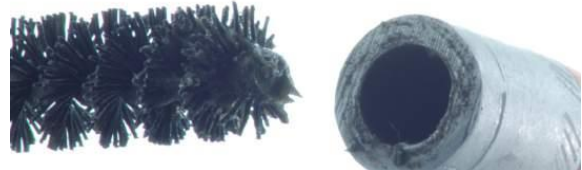
Figure 19: Scrape non-tinned aluminum connectors before use.
