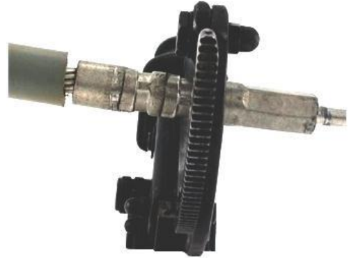
Figure 4: Cut the connector after the top crimp.
