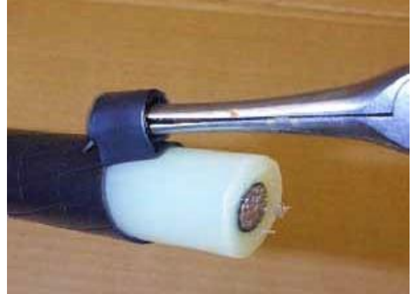
Figure 5: Use pliers to remove the spiral-cut insulation shield.
