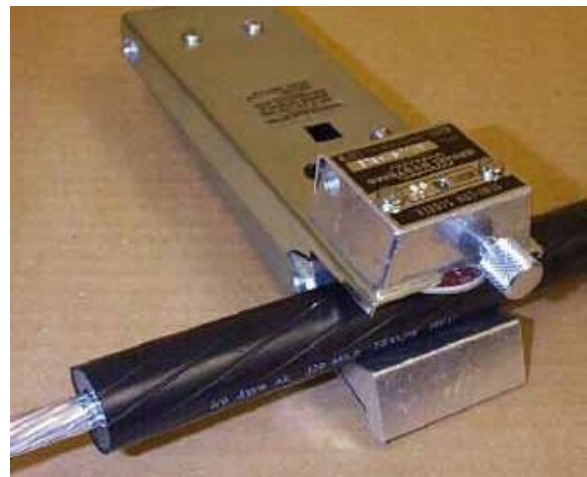
Figure 4: Rotate the tool around the cable to create the square cut first.
