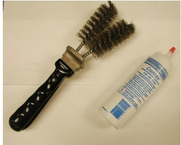
Figure 8: Use wire brushing and corrosion inhibitor to prepare conductor strands for crimping.
